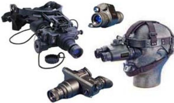
the intensifier tube. The reason green is used is that it is the color most easily seen by the human eye.\* A red phosphor could be applied to preserve night vision of the observer, but it would drain power from the battery at about 100,000 times the rate of the green phosphor!
